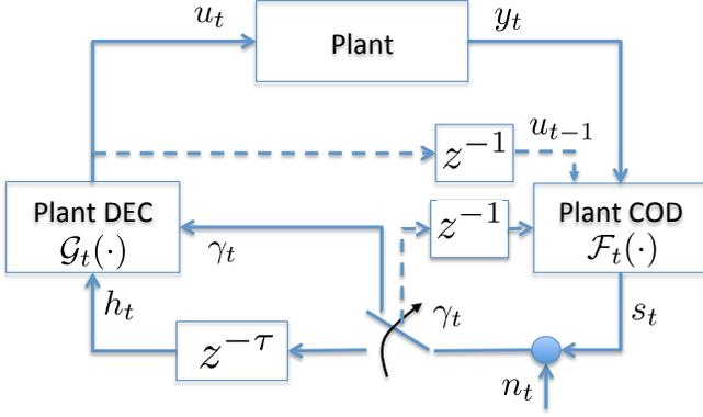
Fig. 3. General scheme of Networked Control System model with implicit channel COD/DEC
