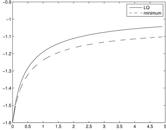
Fig. 5. Comparison between the optimal LQ gain (solid) and the optimal value of  $l$  which solves (23) with cost function  $J$  in (25), (dashed) as a function of  $\rho$  ( $\rho = 0$  corresponds to “cheap control”, i.e. no penalty on the input).
