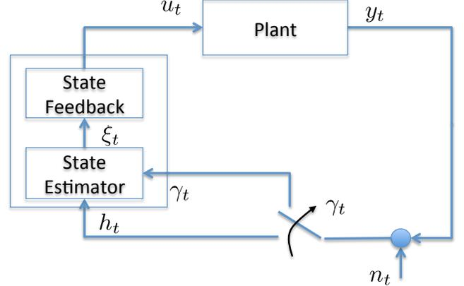
Fig. 4. Special scheme of Networked Control System for scalar output plants
