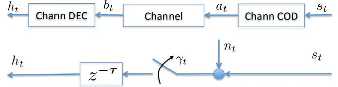
Fig. 2. Equivalent model of Channel COD/DEC using traditional codes
