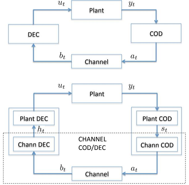
Fig. 1. Scheme of control system across a communication channel: general scheme (top), decoupled scheme (bottom).
